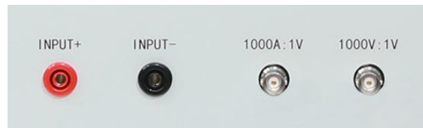
Built-in probe wiring area of the instrument
